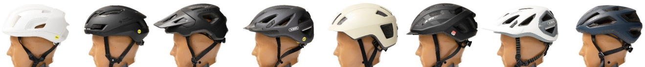
Figure 1. The eight bicycle helmets tested in this study, equipped: MIPS (1–4), KinetiCore (5–6), and EPS-only (7–8).
