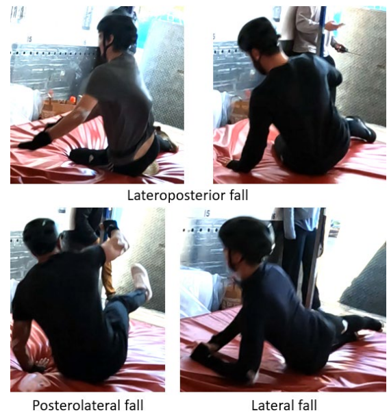
Fig. 2. Fall configurations for specific hip impacts.
