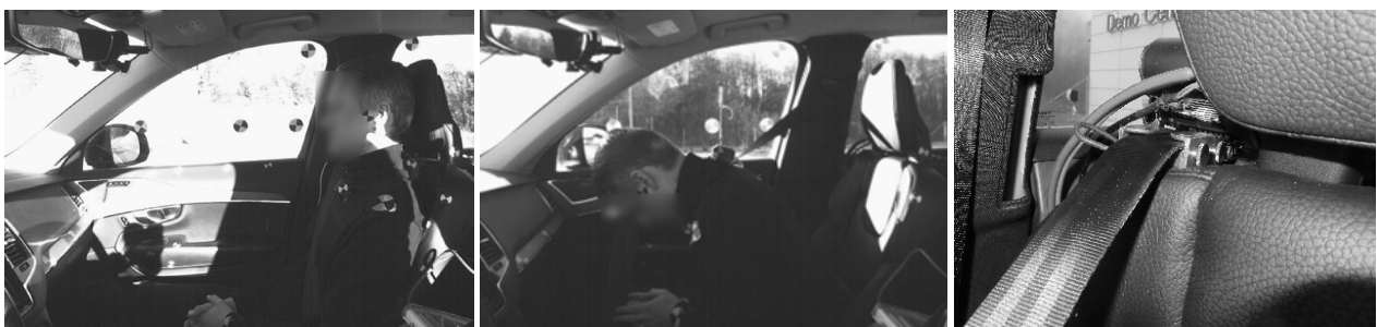
Fig. 1. Upright (left) and forward-leaning (middle) volunteer in the test-vehicle seat, and BIS installation (right).
