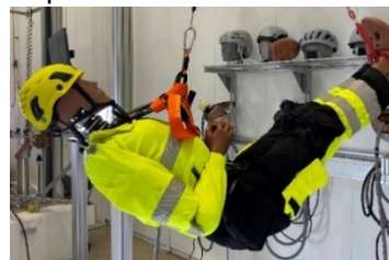
Fig 2. HIII dummy positioned for drop test
