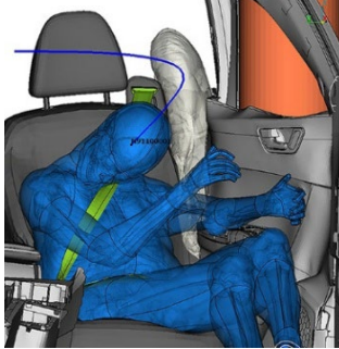
Fig. 2. Head trajectory of the AM50 model in Pole-Sc_0 (maximum DAMAGE/UBrIC values).
