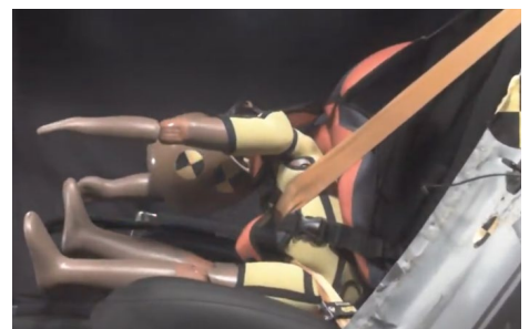
Fig. 5. Product B – side view at 90 ms.
