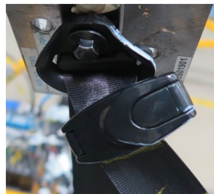
Fig. 10. Detail view of Product F (diagonal belt), which was secured around the diagonal belt in direct contact with the D-loop.
