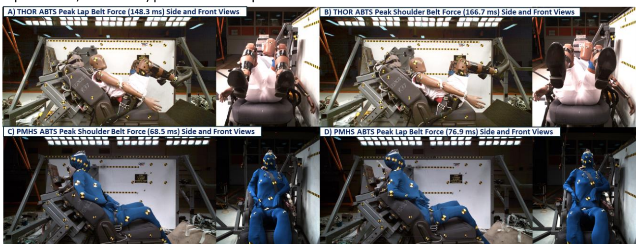
Fig. D9. Comparison of the peak belt loading sequence at 45° recline in the ABTS seat for the THOR-05F and PMHS. For THOR-05F, peak lap belt force (148.3 ms) occurred prior to peak shoulder belt force (166.7 ms). Conversely, the PMHS experienced peak shoulder belt force (68.5 ms) followed by peak lap belt force (76.9 ms).
