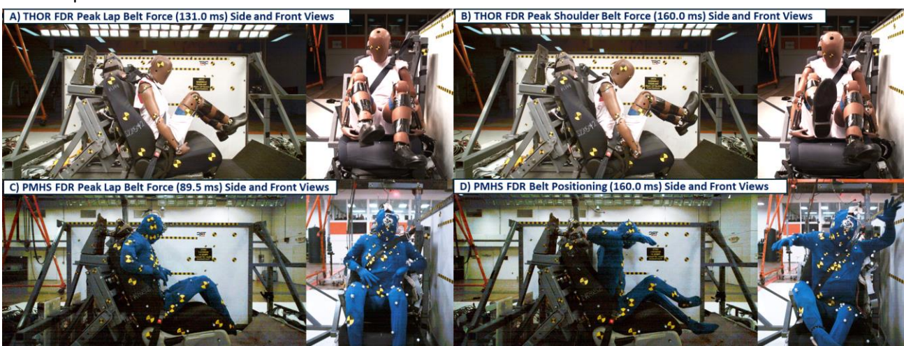
Fig. D4. Comparison of the peak belt loading sequence at 25° recline in the FDR seat for the THOR-05F and PMHS. For THOR-05F, peak lap belt force (131.0 ms) occurred prior to peak shoulder belt force (160.0 ms). For the PMHS, only peak lap belt force data was available, which occurred at 89.5 ms. The PMHS belt positioning at 160.0 ms was included to provide a comparison in the absence of peak shoulder belt data.
