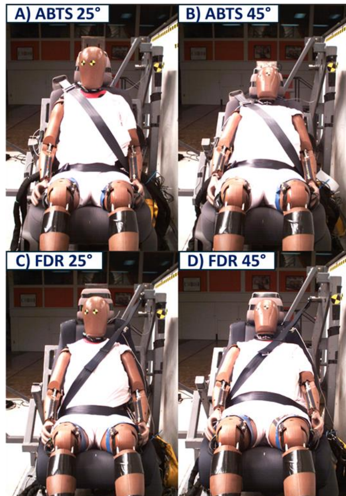
Fig. A3. Fixed recline seatback, fixed head restraint sled test configuration (front view) showing the THOR-05F belt routing in: A) ABTS seat at 25° recline; B) ABTS seat at 45° recline; C) FDR seat at 25° recline; and D) FDR seat at 45° recline. Images are high-speed video stills.
