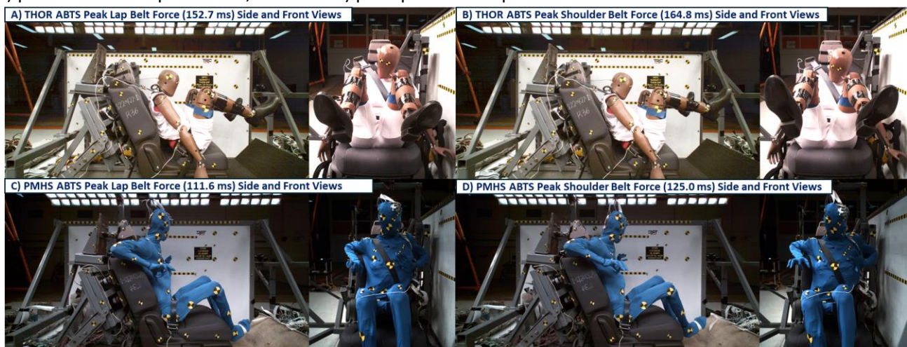
Fig. D3. Comparison of the peak belt loading sequence at 25° recline in the ABTS seat for the THOR-05F and PMHS. Subjects consistently experienced peak lap belt force before peak shoulder belt force. The THOR-05F peaked at 152.7 ms for the lap belt and 164.8 ms for the shoulder belt, while the PMHS peaked at 111.6 ms for the lap belt and 125.0 ms for the shoulder belt.
