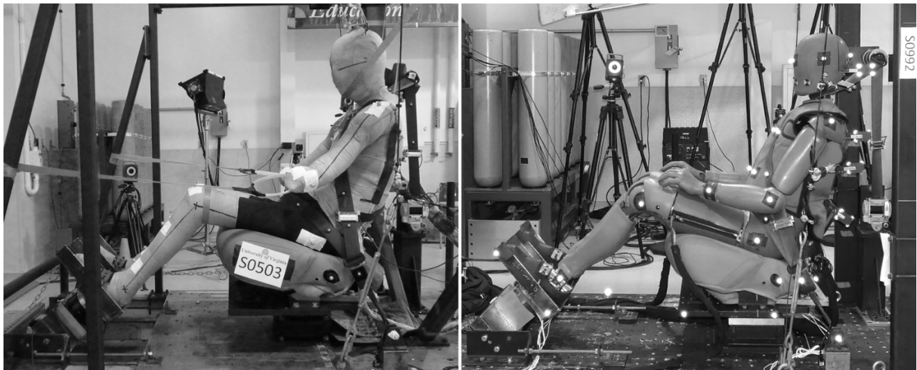
Fig. 2. Left: test fixture featuring a representative mid-size male PMHS (S0503). Right: test fixture featuring THOR-50M-RS (S0992).
