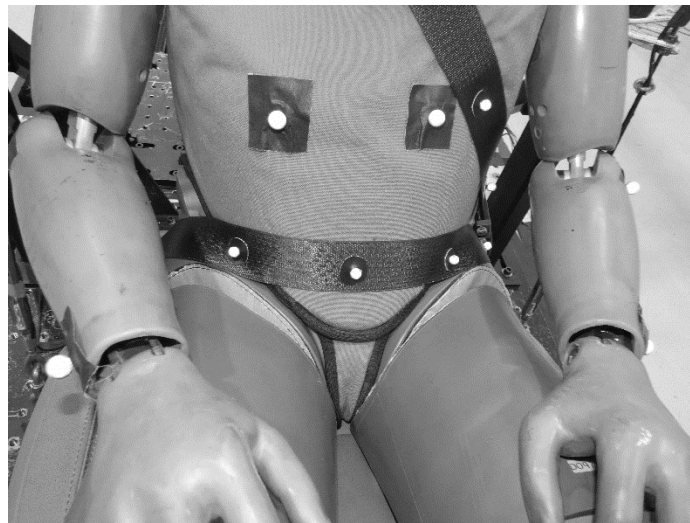
Fig. A2. Lap Belt positioning relative to pelvis and thigh flesh.
