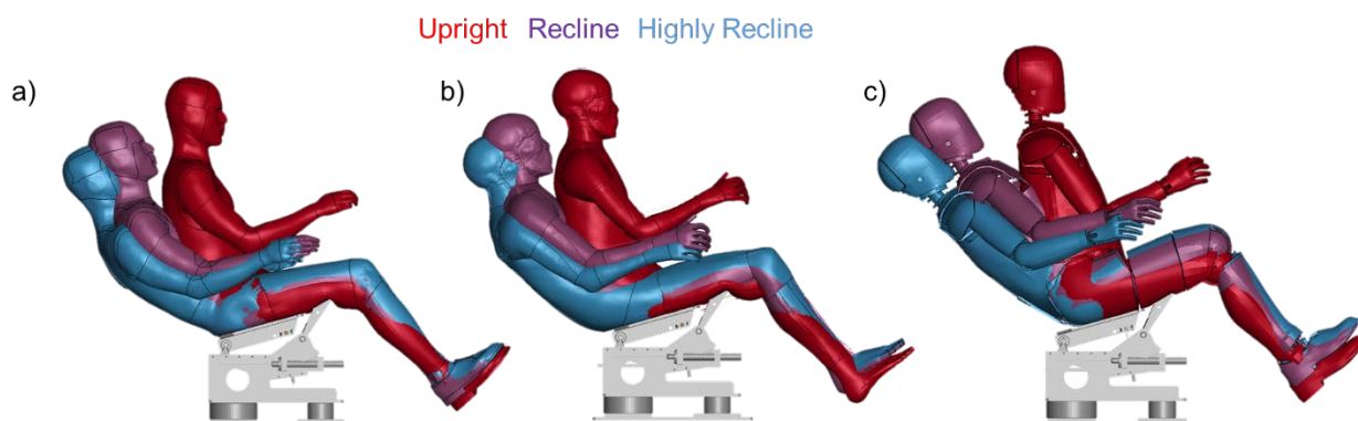
Fig. 1. Example positions for all torso angles for (a) GHBM, (b) THUMS, and (c) THOR.
