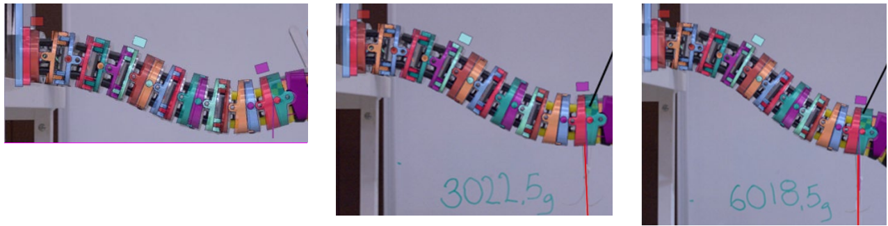
Fig. 4. The loaded state for the three different loadings on the thoracolumbar spine, overlaid with the FE element model under the corresponding quasi-static loading. The cord attached to the spine has been marked with red for clarity.
