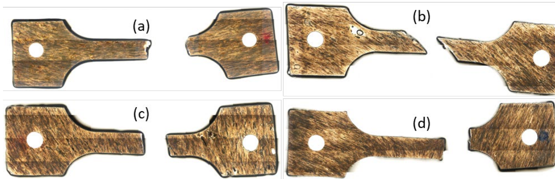
Fig. 8. Exemplar tension coupons with (a) longitudinal, (b) oblique, (c) transverse, and (d) varying osteon alignment with respect to the gage length.
