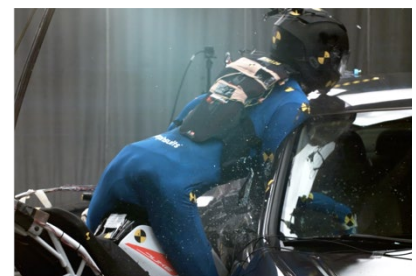
Fig. 5. Exemplar strain data for right and left side anterior ribs (each line is strain from a sperate rib as shown in each legend) and a still frame showing the position of the PMHS at the onset of fracture
