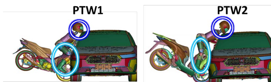
Fig. 27. Comparison of posture of MATD at the head impact between PTW1 and PTW2 for Car5 impact (PTW velocity: 50 km/h, Impact Angle: 90 deg. and Head Impact Location: 0.5).
