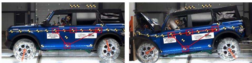
Fig. 1. 2D rigid body tracking methodology. Fiducial marker selection before and during the crash phase.
