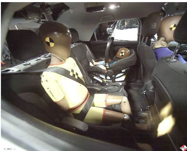
Fig. A 1. Example freeze frames taken at t=0 showing front-row ATDs (top row) and second-row ATDs (bottom row) installed in target vehicles in side impact tests (left column) and frontal offset tests (right column).
