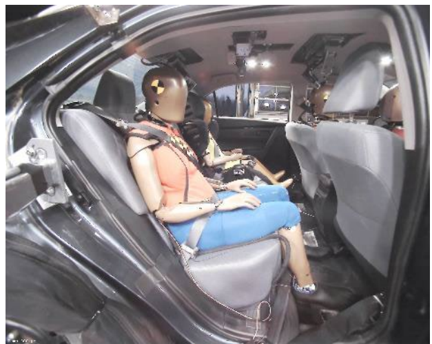
Fig. A 1. Example freeze frames taken at t=0 showing front-row ATDs (top row) and second-row ATDs (bottom row) installed in target vehicles in side impact tests (left column) and frontal offset tests (right column).
