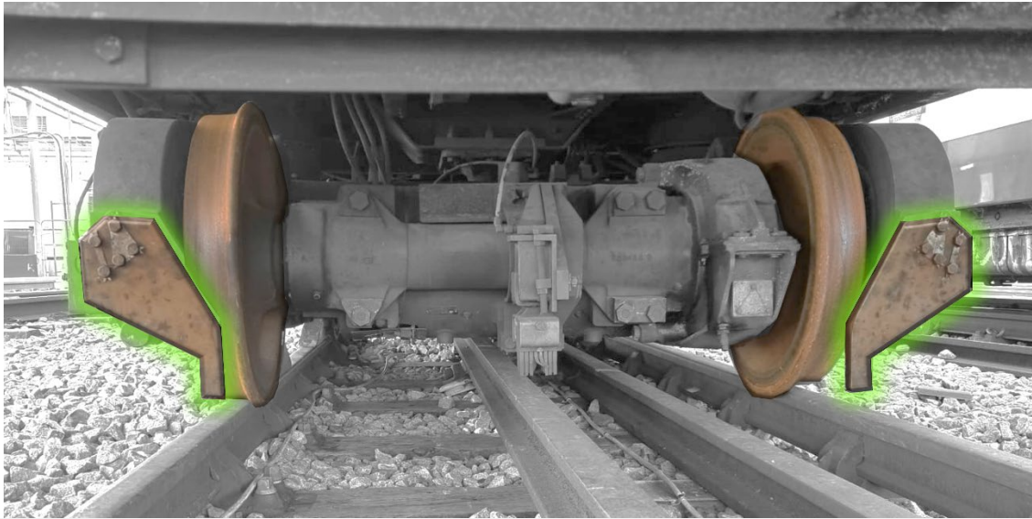
Fig. 1. Train-mounted wheel guard (highlighted) used in London Underground subway cars (image taken by author).
