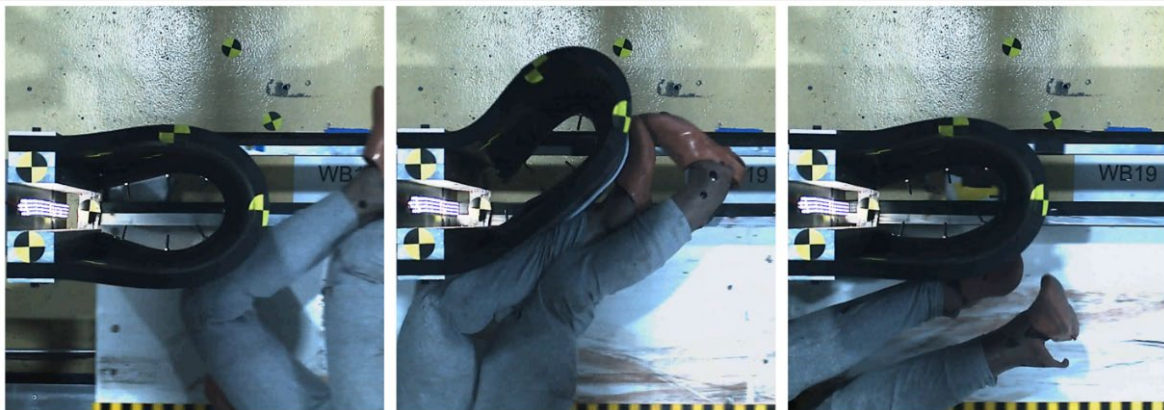
Fig. 6. Lower-extremity kinematics during an 11 m/s (25 mph) impact.
