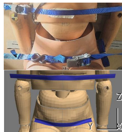
Fig. 2. Restraining heavy-duty cargo strap position for torso and pelvis in experimental testing (top) and in FE environment (bottom)
