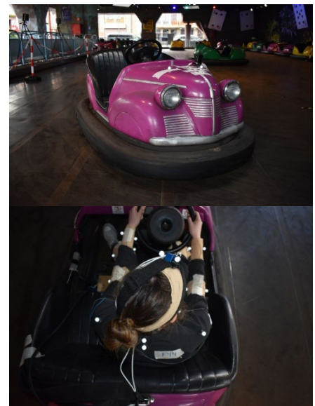
Figure 1a-b: (top) Bumper-car vehicle set-up with VICON markers attached to vehicle and on-board GoPro camera. (bottom) Example test of volunteer rotating head approximately 45° to the right for a rear-end impact.
