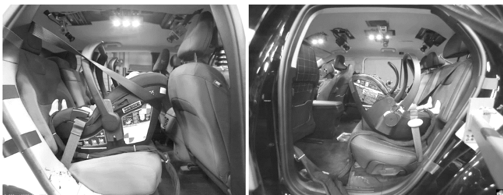
Fig. 1. CRS without a base attached to a vehicle seat using the European (left) and US (right) belt path.
