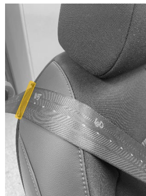
Fig. A2. Location of seatback foam cut. Fig. A3. Simulated integrated belt outlet.
