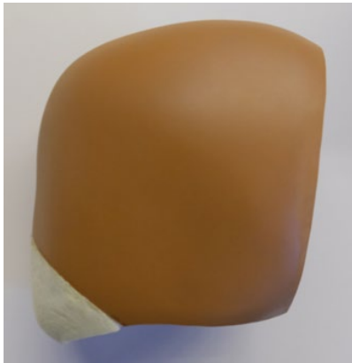
Fig. 1. Cellbond head with soft foam chin element (Q3).
