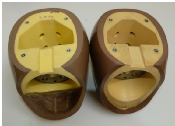
Fig. 3. Humanetics head with skull material removed from the chin (Q3) (left) vs. standard head without modification.
