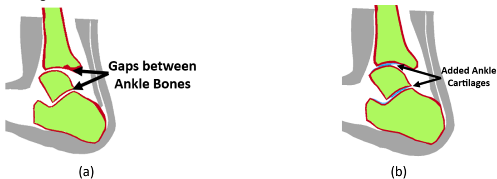
Fig. 2. Cross section of the THUMS AM50 ankle (a) before (b) after addition of the cartilage added to the various articular surfaces of the ankle (highlighted in red color).
