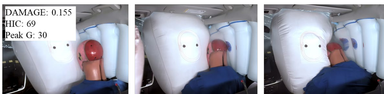
Fig. 4. Passenger-side small overlap right front-passenger head slides off the airbag without linear acceleration or DAMAGE downgrades for the 2021 Chevrolet Traverse.
