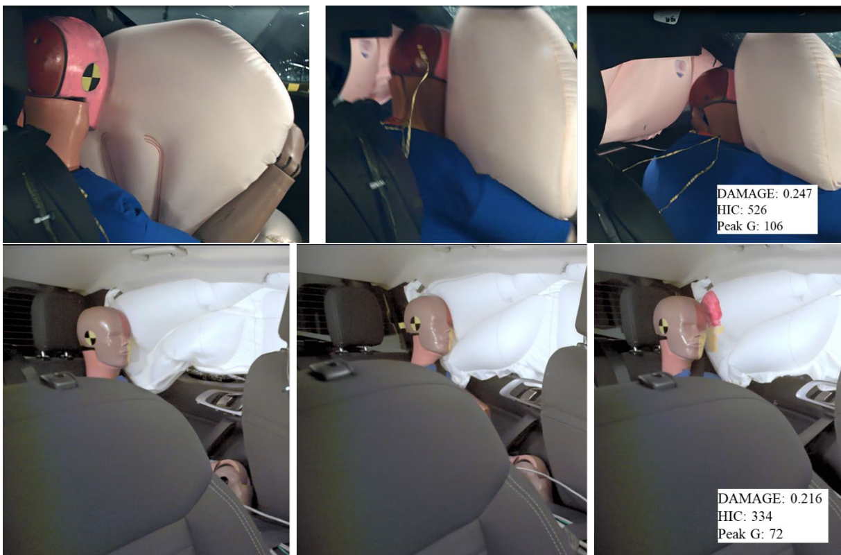
Fig. 2 Examples of peak acceleration downgrades but no DAMAGE downgrades for the 2018 Tesla Model S driver-side small overlap driver ( top ) and 2022 Ford Ranger side impact rear passenger ( bottom ).
