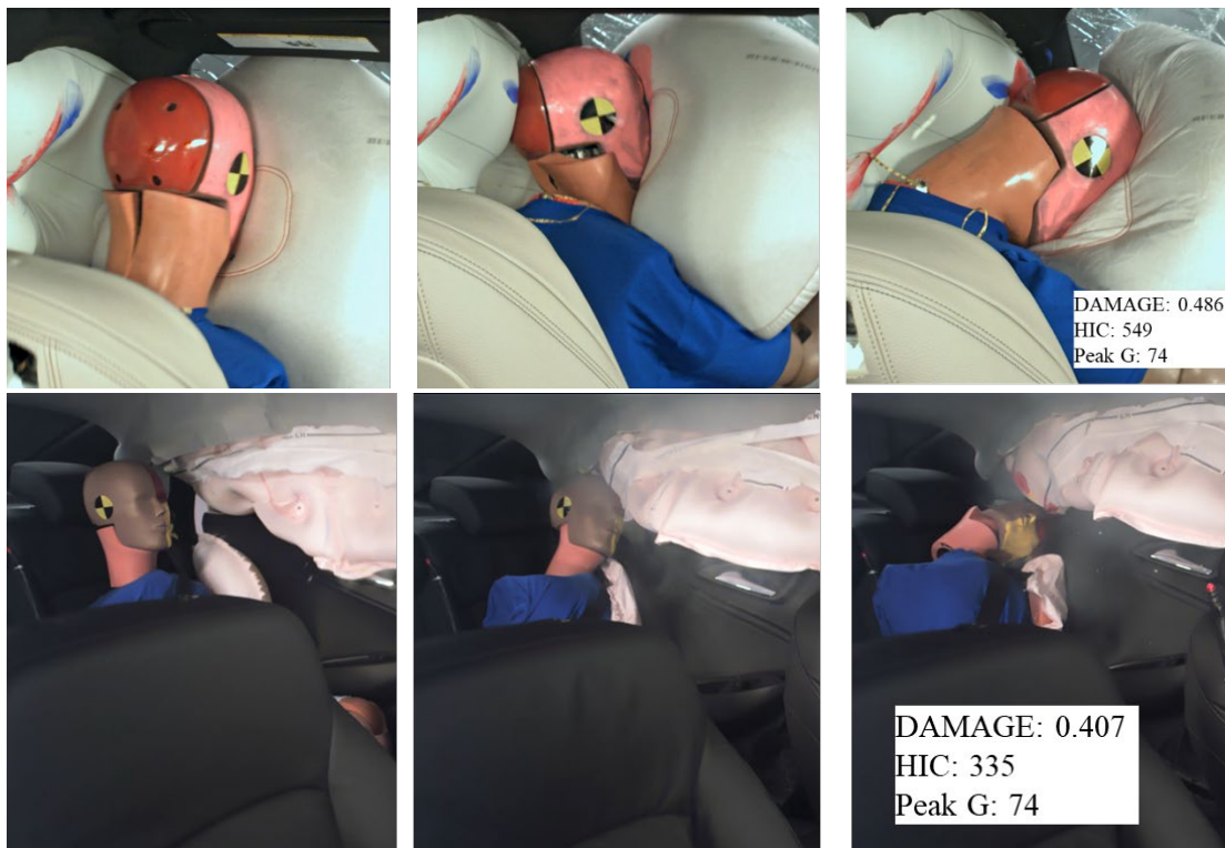
Fig. 3. Examples of DAMAGE and peak acceleration downgrades for the 2017 BMW 330i driver-side small overlap driver (top) and 2022 Chevrolet Malibu side impact rear passenger (bottom).
