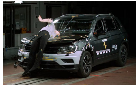
Fig. 4. Dummy position at maximum bonnet deflection during small SUV impact.
