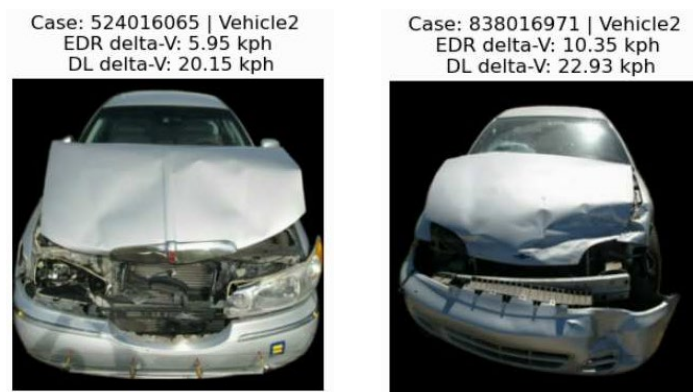
Fig. 12. Hybrid DL model prediction on underride cases.
