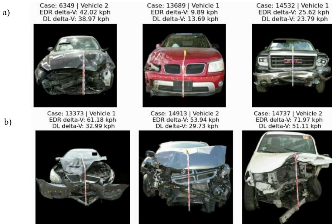
Fig. 11. Hybrid DL model's prediction on a) low severity crashes (< 50 kph), and b) high severity crashes (> 50 kph).
