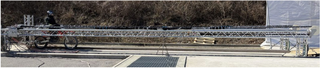
Fig. 7. Catapult ready for a launch: motorcycle/dummy on the carriage, upright posture, bungee pretensioned.
