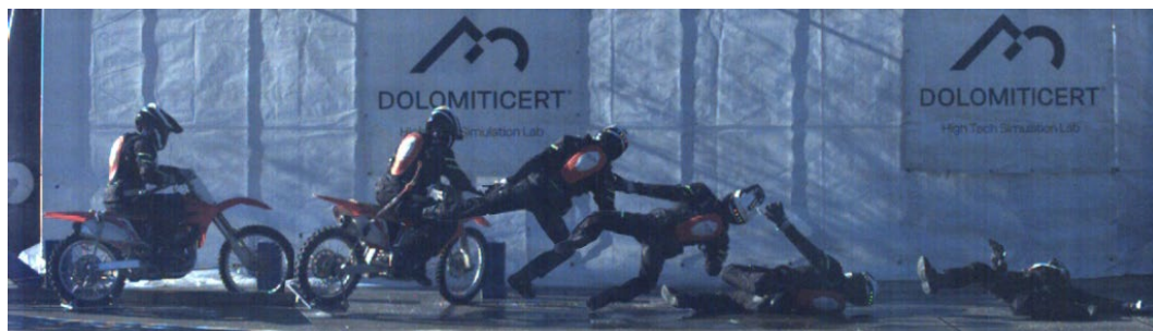
Fig. 17. High side fall physical simulation test example, exit speed 50 km/h.
