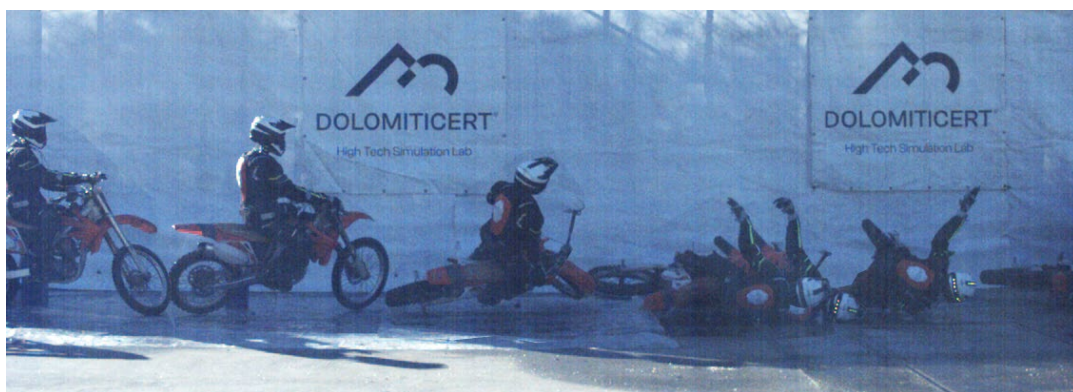
Fig. 18. Low side fall physical simulation test example, exit speed 48 km/h.
