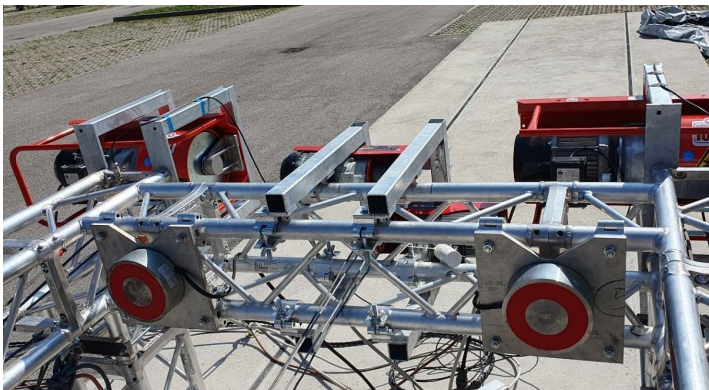
Fig. 5. Catapult rear beam with central recall winch and two electromagnetic anchors.
