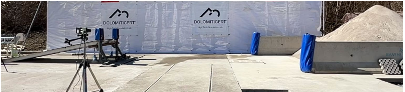
Fig. 8. Setup for jump landing crash simulations with ramp and landing sand pile.
