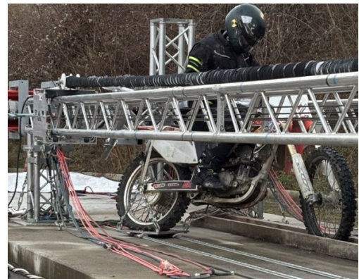
Fig. 6. Catapult ready for the high side fall simulation launch: motorcycle/dummy on the carriage, bungee pretensioned, stopping ropes connected.
