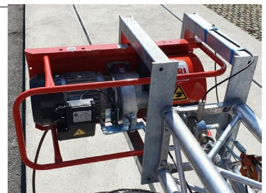
Fig. 4. Bungee rear pretension winch and control load cell.
