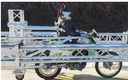
Fig. 2. The carriage launching and support system.
