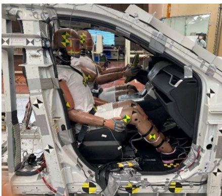
Fig. 2. Overview of dummy installation (Sled test 2).
