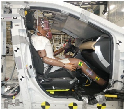
Fig. 1. Overview of dummy installation (Sled test 1).
