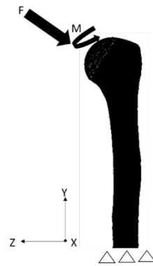
Fig. 2. Coordinate system and Loading Conditions.
