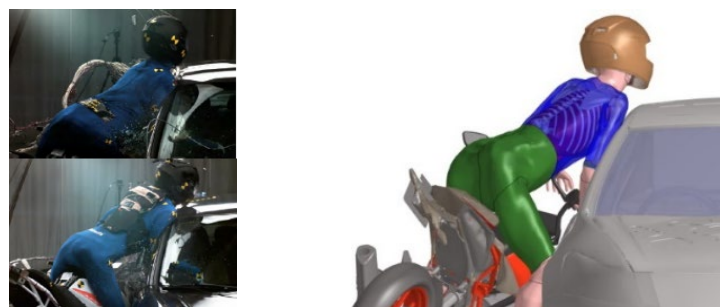
Fig. 3. Images from two KTM 390 crash tests with PMHS [9] (left) and reference simulation (right) moment before thorax impact.
