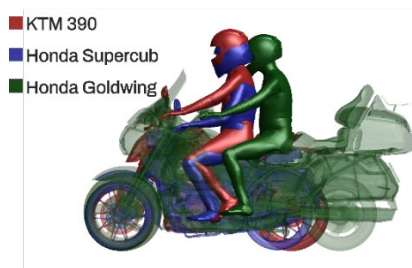
Fig. 2. HBMs positioned on three FE motorcycle models.
