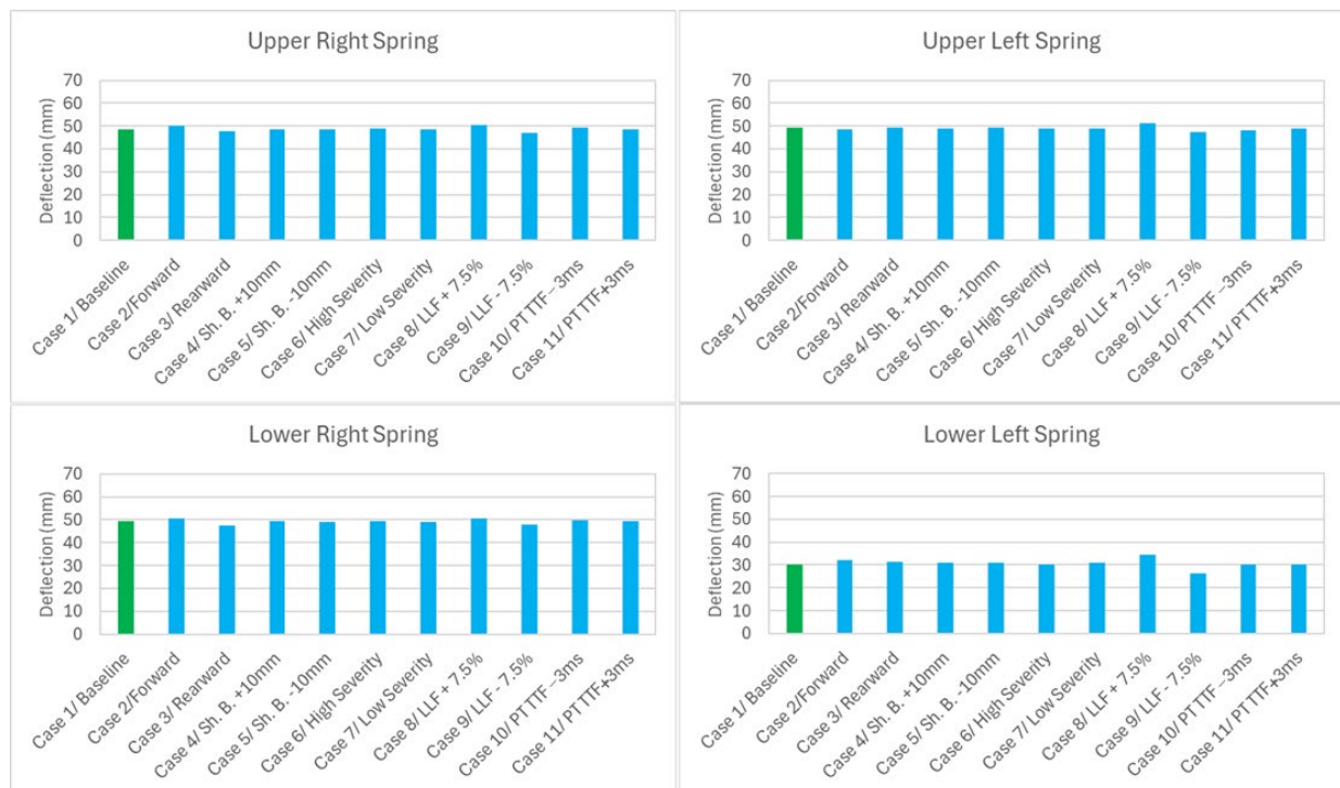
Fig. B1. Comparison of chest deflection in HBMC50M across all simulated cases with the baseline case. These deflections from four locations correspond to the four IR-TRACC locations in THOR50M.
