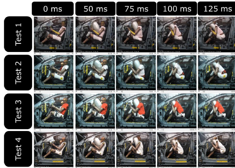
Fig. 1. Driver THOR-50M dummy kinematics showing consistency among all four tests.
