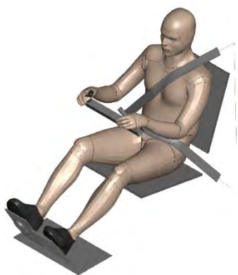
Fig. 1. Simulation setup for simulating pre-crash braking and low-speed impact events using M50-OS+Active.
