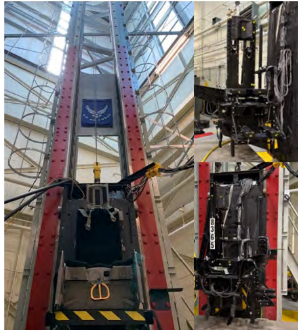
Fig. 2. VDT and experimental seat.
