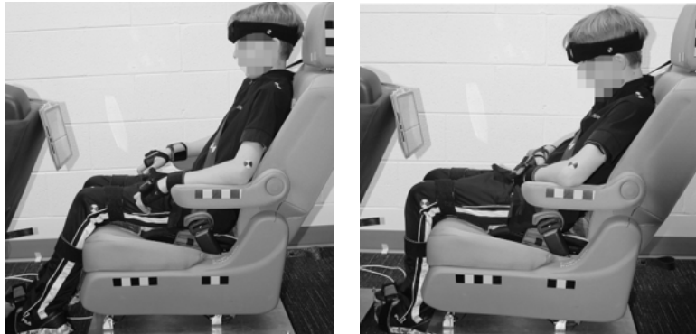
Fig. 2. Exemplar subject in the upright, ideal, reference posture (left) and a self-selected comfortable posture assumed naturally during the 30-minute trial (right).
