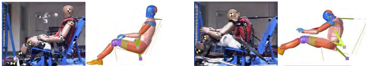
Fig. 4. Kinematics of THOR-AV in sled test and simulation at 0ms (left) and the moment of maximum pelvic forward excursion (right).
