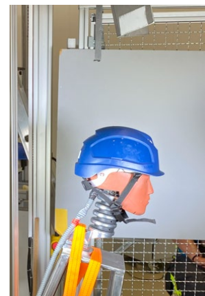
Fig. 1. Test set-up, with HIII head and neck and the drop-slide.
