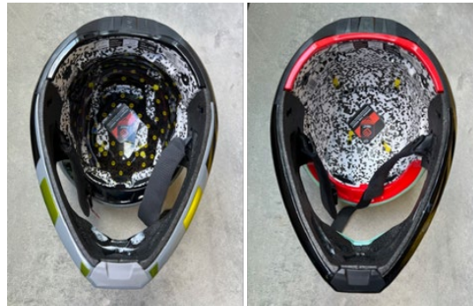
Fig. 3. MX helmet tested with (left) and without (right) rotational mitigating technology.
