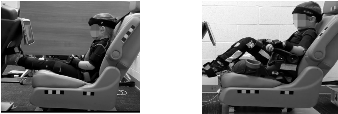
Fig. 6. Examples of how volunteers modified their posture to support their feet along the back of the front captain's chair (left, baseline configuration), and on the front edge of the seat pan (right, high-profile configuration).
