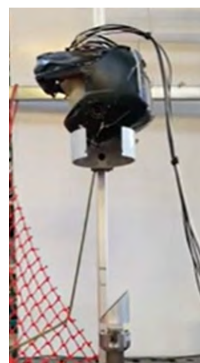
Fig. 5. Experimental rig for protected impact tests performed onto the 45° inclined anvil using the IHHR from 1 m.
