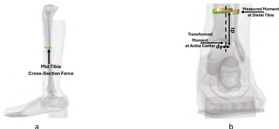
Fig. 6. Model instrumentation a) cross-section force at mid-tibia b) the moment at the ankle joint center calculated via transformation of the forces and moments measured in the distal tibia and fibula.
