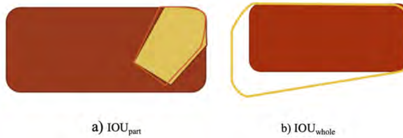
Fig. 5. Illustration of IOU Part versus Whole, highlighting the distinction in bounding box overlap assessment [43].
