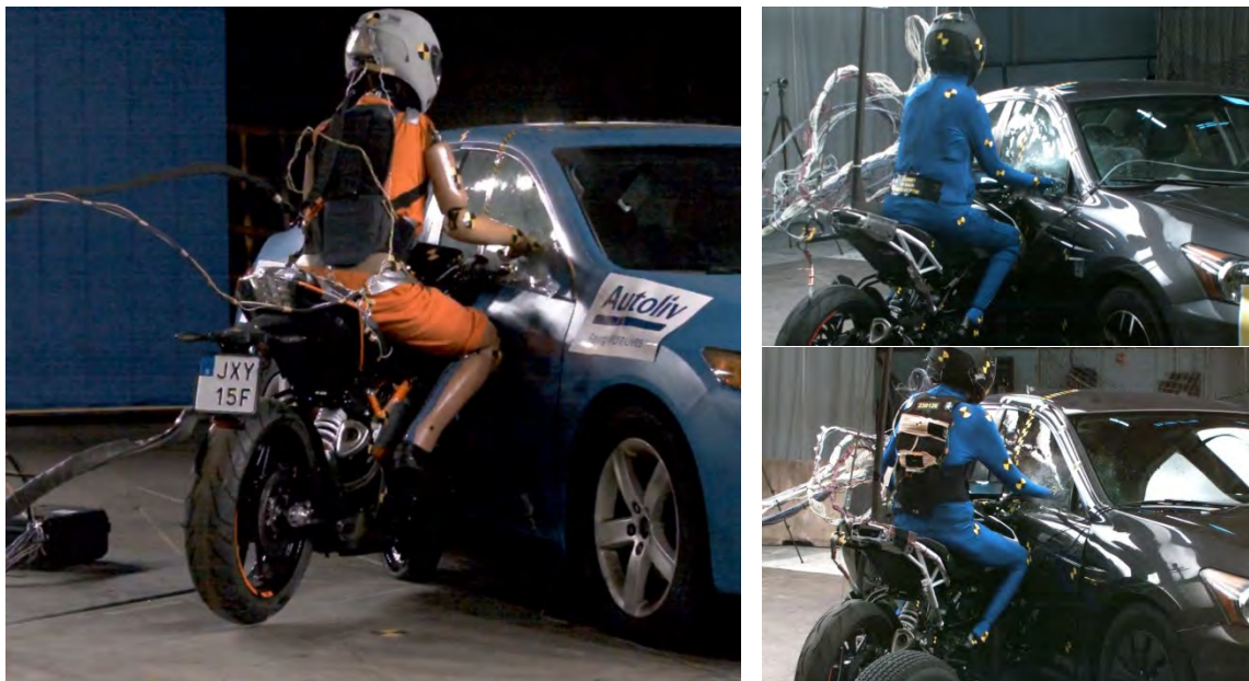
Fig. 6. Still images showing the moment of pelvis contact with the fuel tank (PTW Dummy left, PMHS right).
