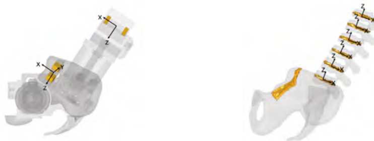
Fig. 3. Cross section definitions for lumbar spine vertebra L1 and pelvis iliac wing of THOR-AV (left) and THUMS (right). Intervertebral discs not shown for the lumbar spine of THUMS.
