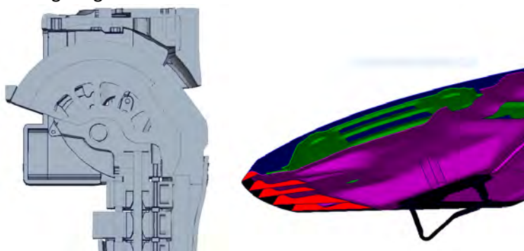
Fig. 2. Implementation of ribs (red) between the exterior and interior sheet (full section at Y0).
