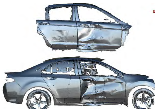
Fig. 3. Images from scanned post-test car side-profiles of the Honda Accord from the second PMHS test (American),
