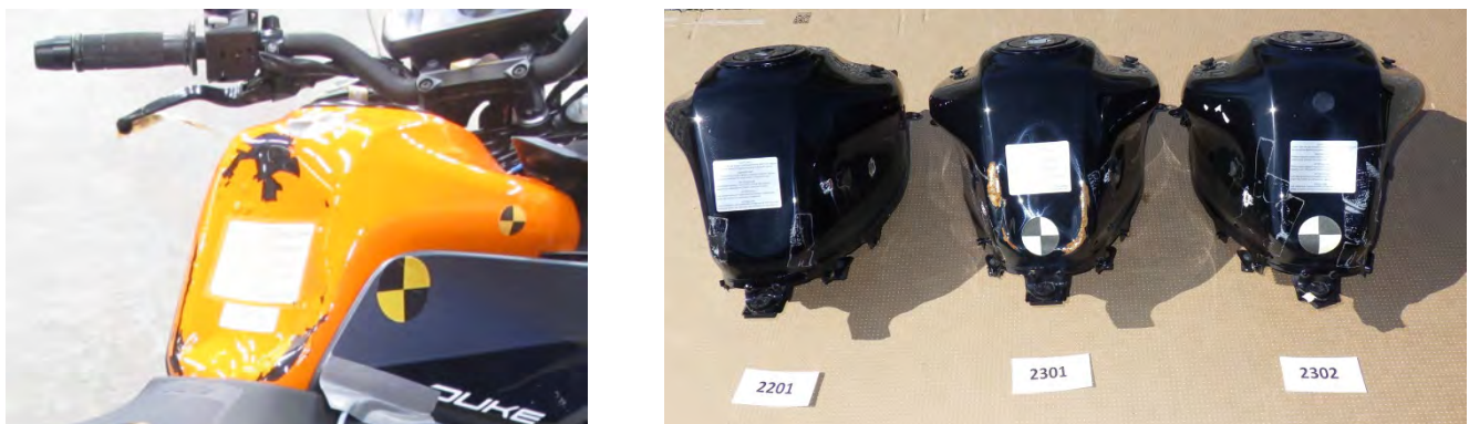
Fig. 7. Images showing the deformation of the fuel tank from the PTW Dummy test (left) and the three PMHS tests (right).
