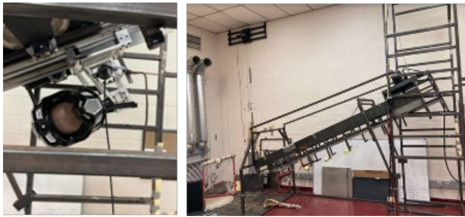
Fig. 1. Rail-guided launcher (RGL) used for all head impacts. Consists of adjustable rails and a steel carriage to anchor and guide the headform.
