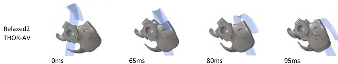
Fig. 7. The motion of the lap belt and pelvis in the submarining case.
