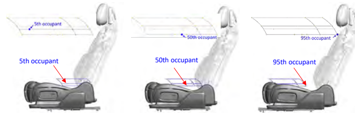
Fig. A3. Seat positions for the 5 th , 50 th and 95 th occupants.
