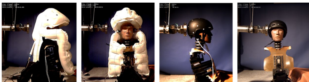
Fig. 1. Experimental setup for the rear and side head impacts with the airbag and with the helmet.
