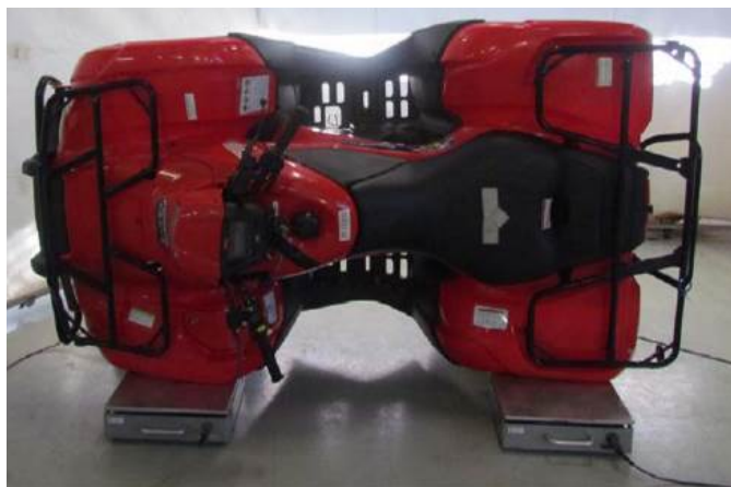
Fig. 5. Contact force tests measured using load scales.
