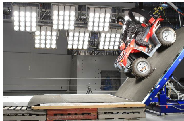
Fig. 8 Dynamic rollover test, forward pitch roll just prior to release, quad bike with lifeguard OPD (G140085).
