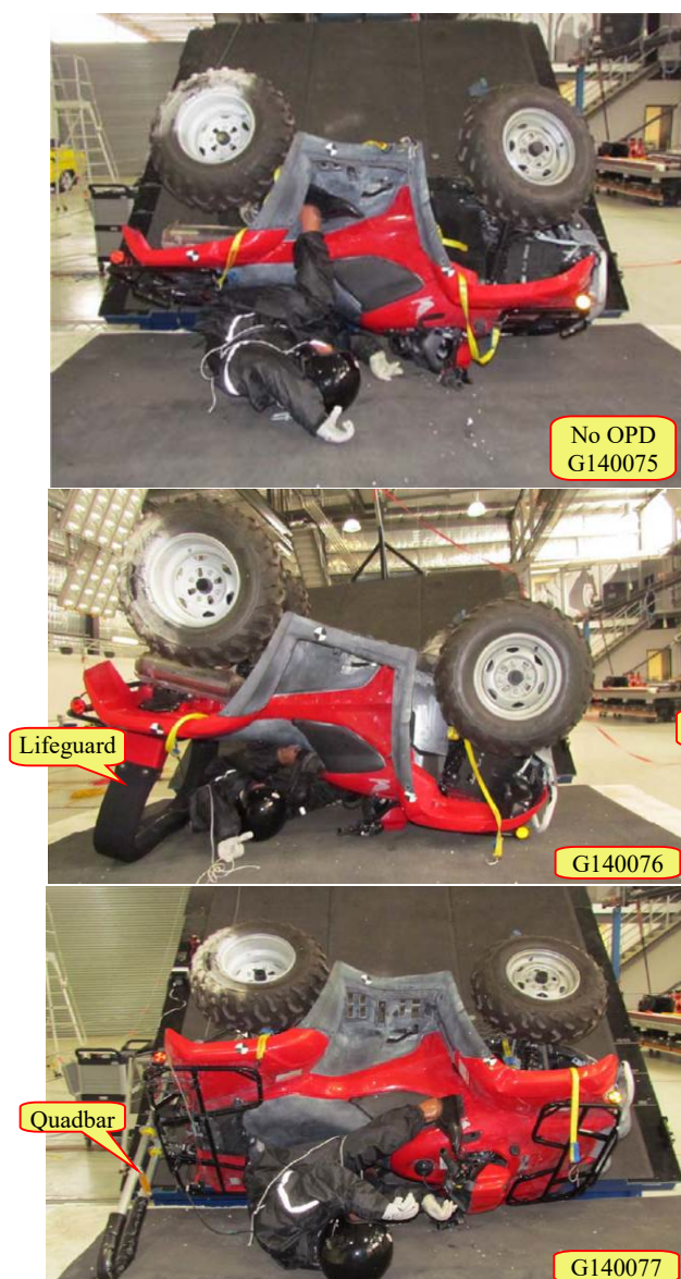
Fig. 12. Lateral rollover: top - no OPD; middle - with Lifeguard OPD; bottom – with Quadbar OPD.
