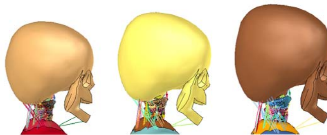
Fig.4 - The 1.5 y.o (left) and 6 y.o models (right) obtained by scaling using the PIPER Kriging tool and the Kriging net reported in Figure 3. The head model has been attached to a new neck model developed as an effort in the PIPER European project (just for visualisation).
