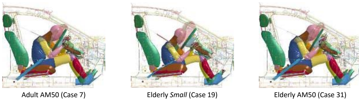
Figure 3. Body kinematics for three driver models (Adult AM50, Elderly Small , and Elderly AM50) with a 4kN belt force limit and Mid airbag setting
