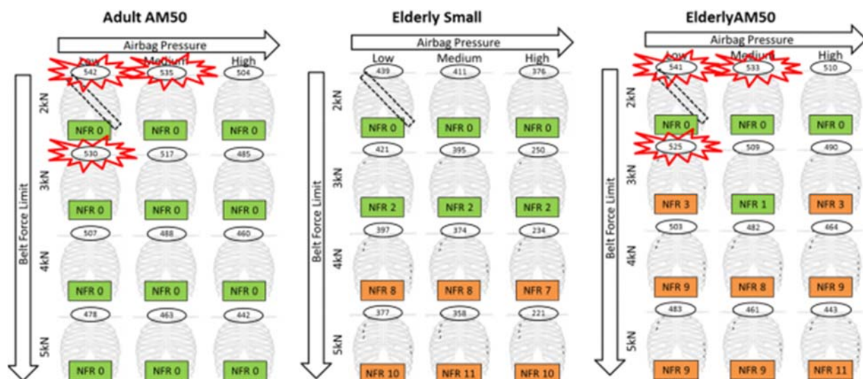
Figure 9. Number of fractured ribs and peak head forward displacement for all occupant and restraint systems settings presented in this study. Head strikethrough cases are highlighted with a red sign.
