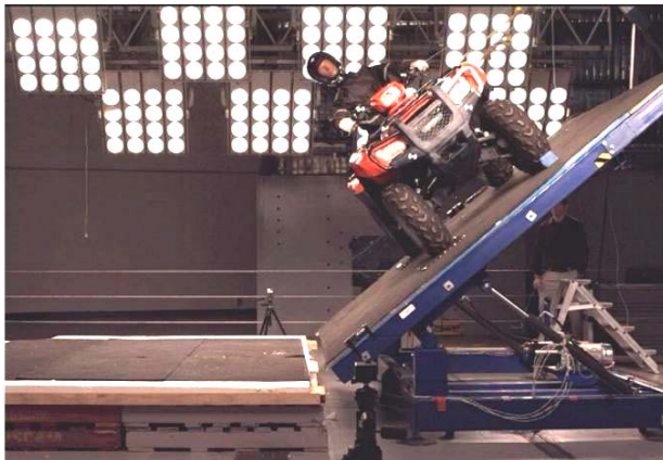
Fig. 7 Dynamic rollover test, lateral roll just prior to release, quad bike with no OPD (G140075).
