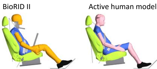
Fig. 5. Simulation set-up of rear-impact test 1: seat 1, with head restraint in nominal position and occupant in nominal position.
