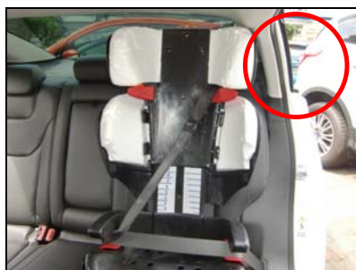
Fig. 11. No full height adjustability possible due to contact between CRS and C-pillar in a large family car.
