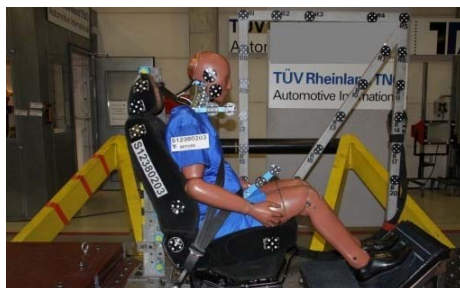
Fig. 1. Initial position of rear-impact test 5 with seat 1, lowest head restraint position and BioRID II bent forward.
