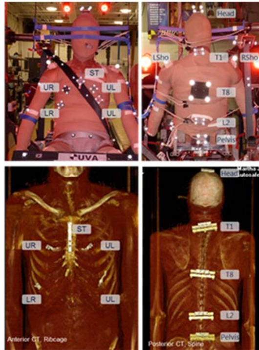
Fig. 3. Subject motion capture measurement hardware.
