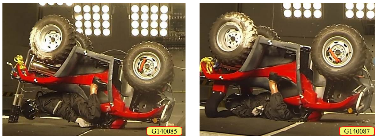
Fig. 16. Forward pitch roll over test showing how OPD interacts with MATD head and neck.
