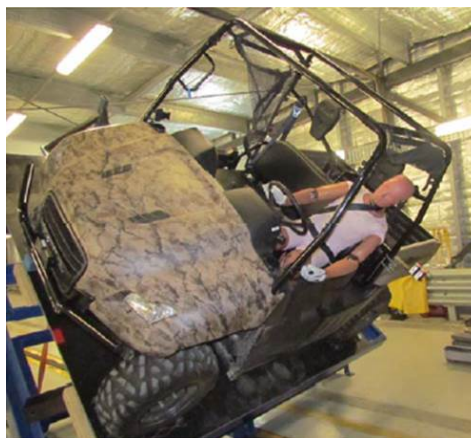
Fig. 6. Occupant retention tests using tilt table
