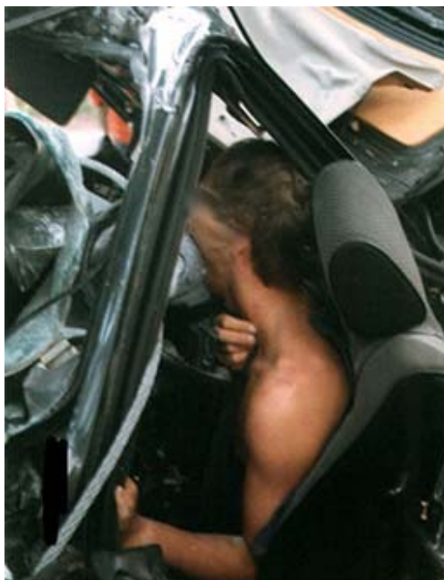
Fig. 17. Example of dislocation of the steering column after frontal car collision, accident year 1991.
