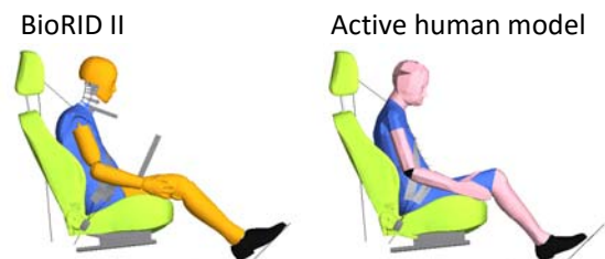
Fig. 6. Simulation set-up of rear impact test 9: seat 2, with head restraint in highest position and occupant in bent forward position.
