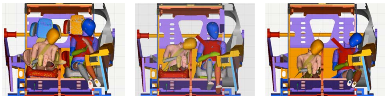
Fig. 12. Kinematics at 75 ms of all dummy-CRS combinations of the initial pulse. Left : CRS with back rest; middle : with booster cushion; right : without CRS.
