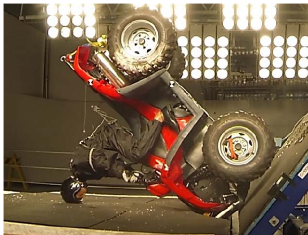
Fig. 11 Forward pitch test (G140088) demonstrating how rider can receive serious cervical spine injury. MATD neck was fractured twice during testing.
