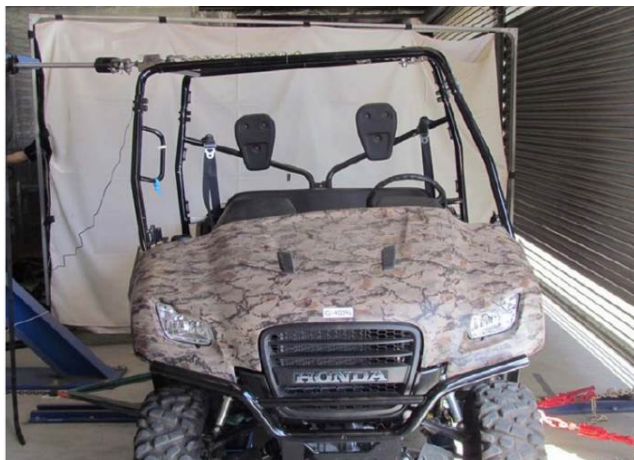
Fig. 9. Honda Big Red SSV subjected to lateral loading. Fig. 10. Honda Big Red SSV subjected to vertical loading. located on each side of the vehicle. The two cylinders pulled down on a flat rigid steel load plate that was positioned to cover the top surface of the ROPS.
