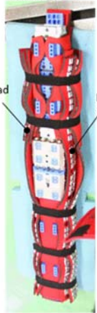
Fig. 5. Overview of the lower limb part of the aPLI PT actual test tool (flesh).
