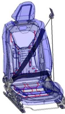
Fig. 2. Prototype Seat FE Model.
