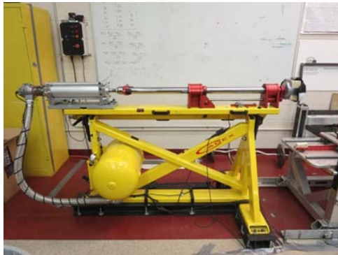
Fig 1. Linear impactor used for the adult collisions with the impact cap that simulated the compliance of a shoulder.
