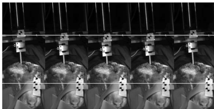
Fig 3. Impact sequence of Sheep B. Frames separated by 15 ms. The two horizontal lines indicate stationary positions of the indentation rod (upper line) and the sheep head (lower line). The motion of the indentation rod is indicated by the movement of the upper target. The sheep's head remains stationary during the impact as indicated by the stationary position of the lower targets.
