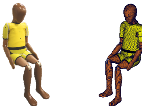
Fig. 1. Q10 dummy and equivalent finite element model.
