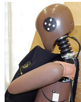
Fig. 6. Side impact kit installed on the dummy.
