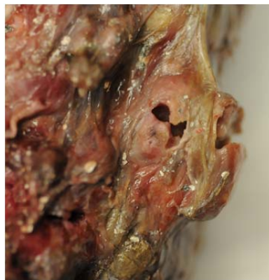
Figure 6. Post-test dissection showed a failure in the osteophyte bridging the C4 and C5 vertebral bodies as well as disruption in the ALL.
