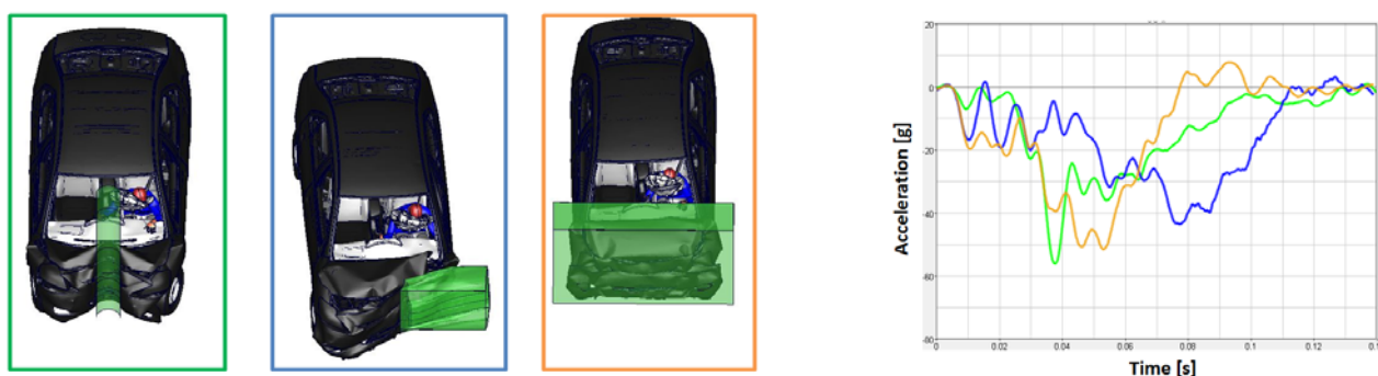
Figure 11 – Integrated occupant vehicle model with THUMS (left) and vehicle pulses (right) in Center Pole (green), IIHS (blue) and NCAP (coral) load case
