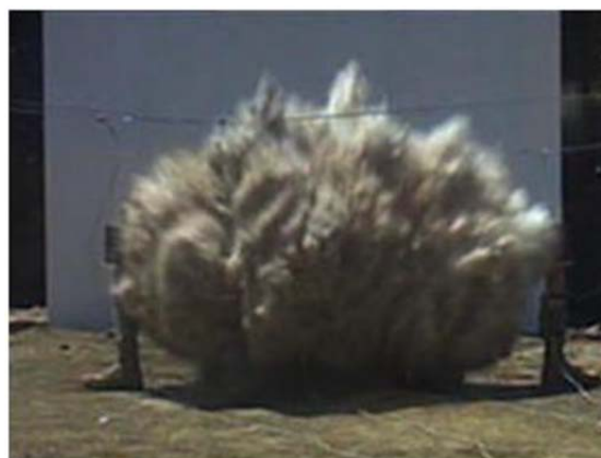
Figure 15. A frame from the high-speed video demonstrating that the soil ejecta cloud radiates out of the ground over the center of the charge. The interaction of the cloud and the leg in this experiment occurs along the tibial shaft, which is unlike the loading conditions from the previous landmine experiments where the leg is directly over the charge.
