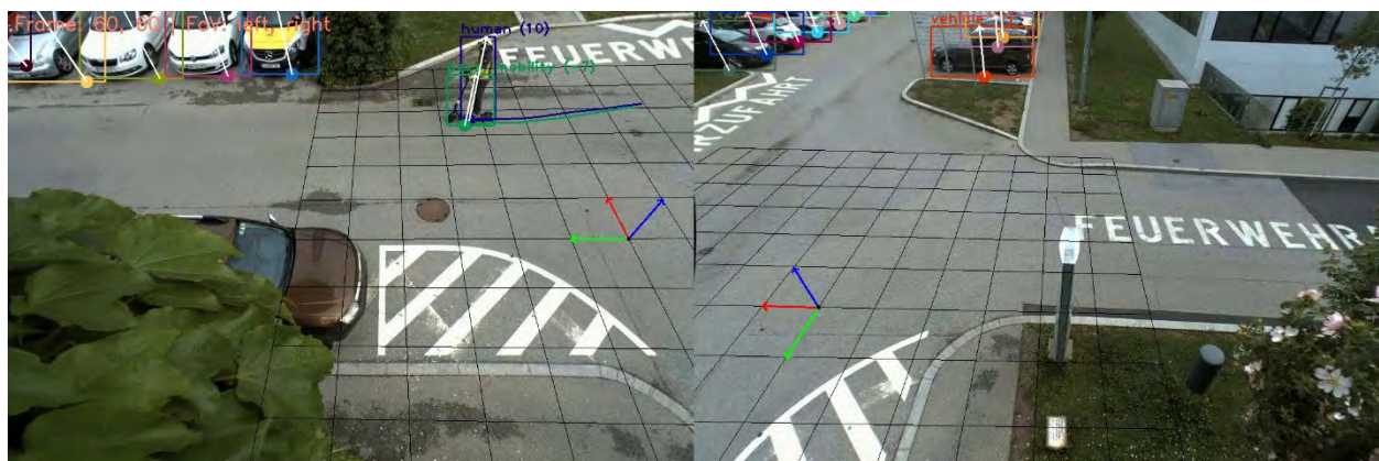
Fig. 1. Left and right field of view of the installed observation system, which is capable of detecting and tracking humans in the recorded video sequences. Coloured bounding boxes and trajectories correspond to the object's ID. The white coloured orientation vector estimated the volunteer's foot point, which was used for trajectory reconstruction. The left image shows the projected trajectory onto ground plane, defined by the extrinsic camera calibration. The coordinate system, which has been aligned with a road network model is illustrated via arrows pointing along the major axes (red: X-axis, green: Y-axis, blue: Z-axis)
