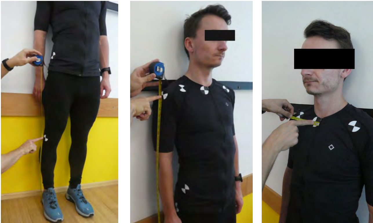
Fig. A1. Determination of height of knee, trochanter, shoulder with respect to the floor level. Collarbone is measured to the mid-sagittal plane.
