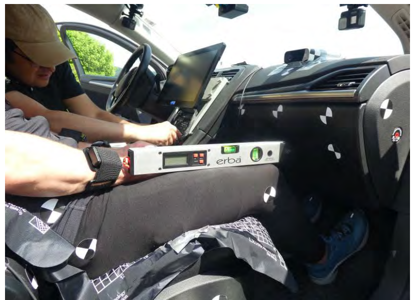
Fig. A4. Position of the seat belt in relation to the collar bone (body centre).
