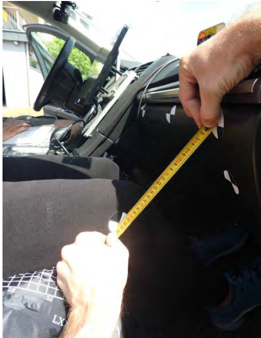
Fig. A3 Position of knee and trochanter relative to vehicle interior markers.
