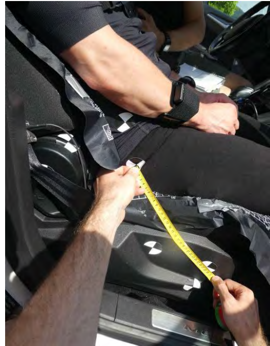
Fig. A3 Position of knee and trochanter relative to vehicle interior markers.
