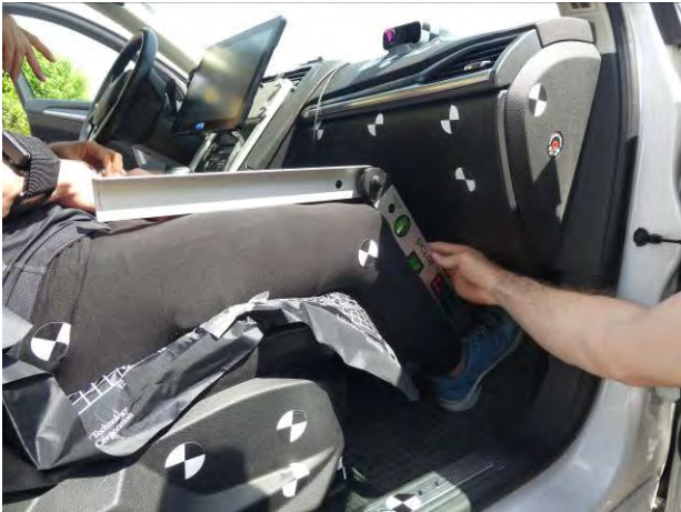
Fig. A6. Angle between upper / lower leg and angle of the Frankfurt plane.
