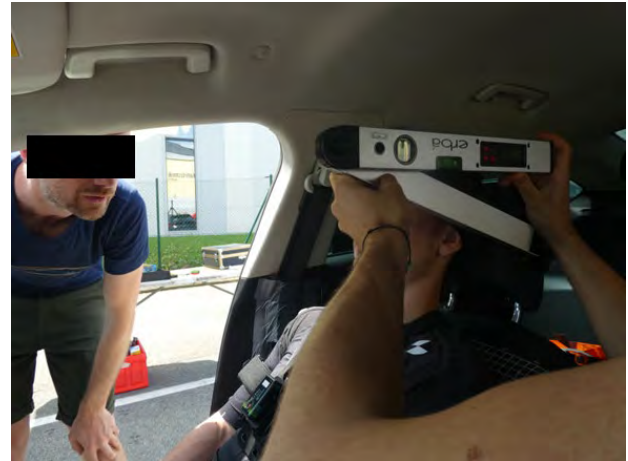
Fig. A6. Angle between upper / lower leg and angle of the Frankfurt plane.
