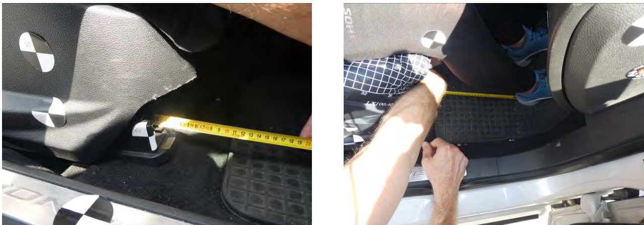
Fig. A2. Longitudinal position of the seat and position of the heel relative to the seat rail.
