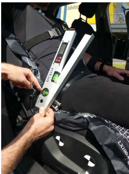
Fig. A4. Position of the seat belt in relation to the collar bone (body centre).
