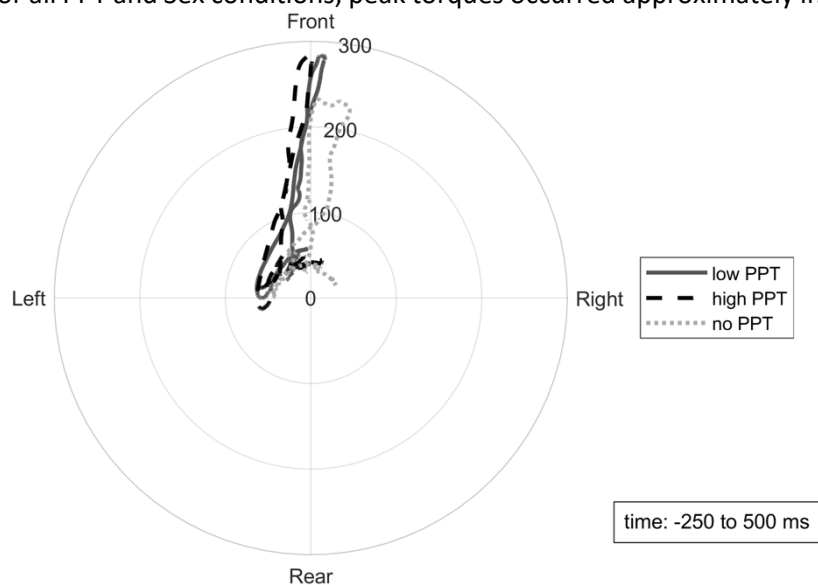
Fig. 4. Polar plot indicating direction in the plane of the seat pan and magnitude (Nm) of the torque applied to the seat over the duration of the frontal impact tests, separated by PPT condition, for the 16 adult subjects.
