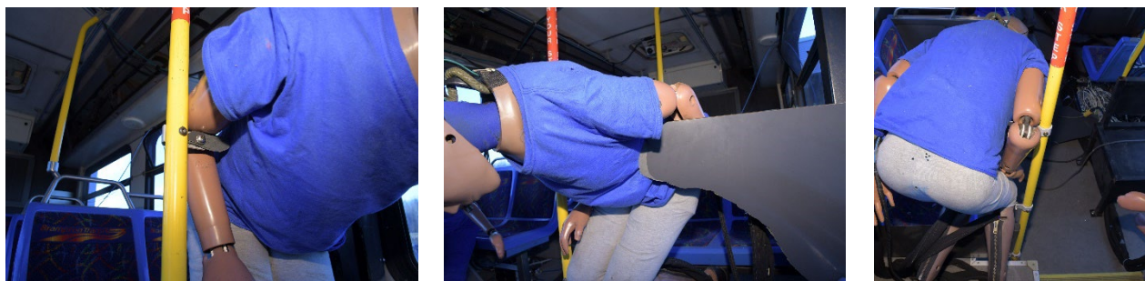
Fig. 12. Post-test photos of final positions of the Hybrid III 5 th percentile interaction with barrier hardware.
