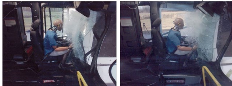
Fig. 7. Freeze frames of the driver ATD at peak head excursion in Test 3 and Test 4 (pair of New Flyer B40 LF buses with and without reinforcement).
