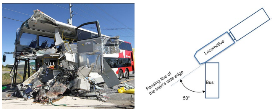
Fig. 1. (Left) Photo of damage to the bus and (right) schematic of the 2013 collision between a bus and a passenger train.
