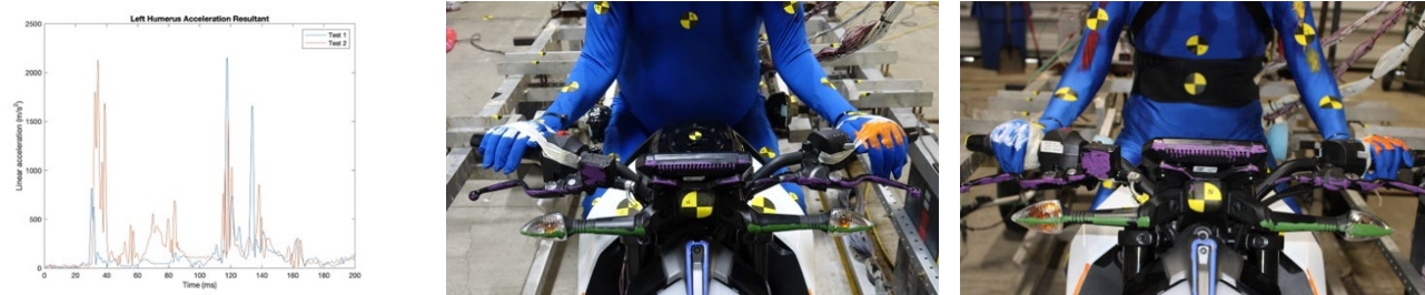
Fig. 4. Resultant left humerus acceleration for Test 1 and Test 2, a still photo from Test 1, and a still photo from Test 2.
