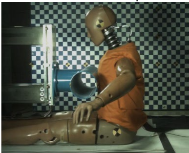
Fig. 1. HIII-50M in position before linear impactor loading to the thorax.
