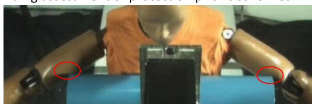
Fig. 3. Wide impactor-to-arms contact (red) shows the need for a maximum impactor width.
