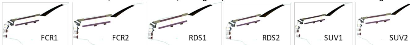
Fig. 2. Shape-matched buck models of three vehicle categories.
