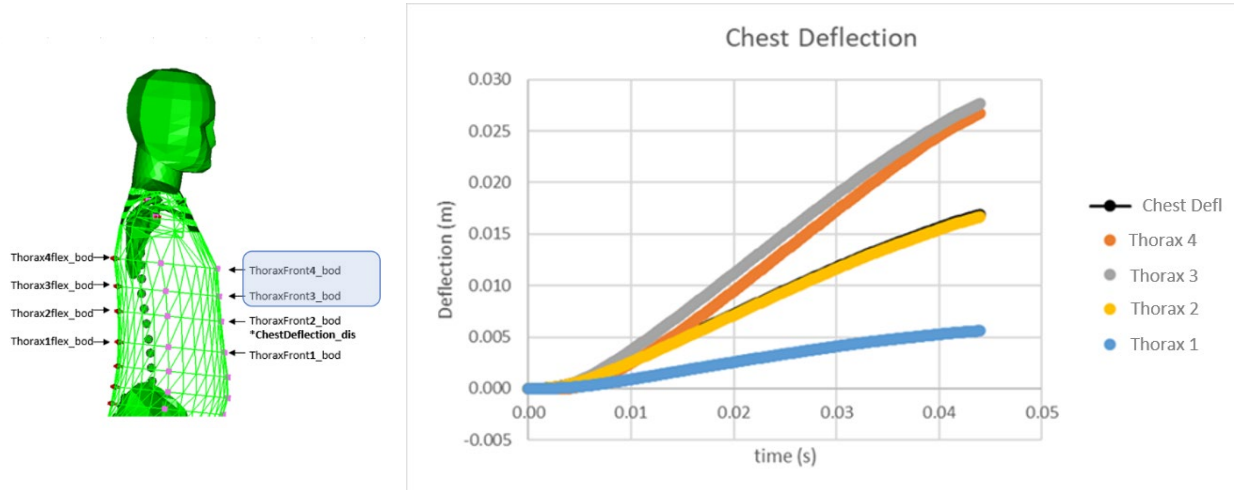
Figure 2 shows the chest deflection time history at the 4 chest deflection measurement locations (all located on the mid-sagittal plane). Each level shows different amount of chest deflection, with the Thorax3Front_bod being the highest.
