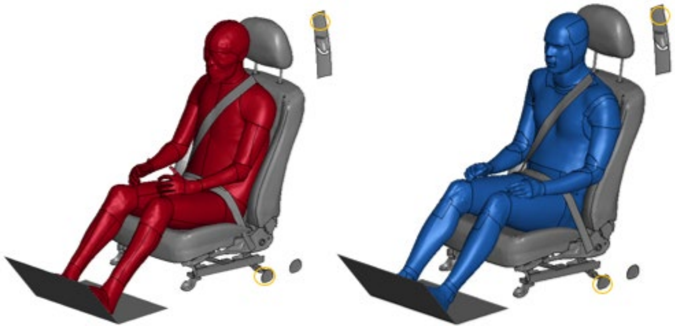
Fig. 3. HBM position in seat and belt retractor locations.
