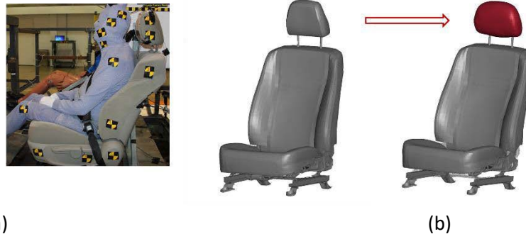
Fig. B1. Matching the head restraint geometry of the FE seat to the physical seat: (a) 2011 Toyota Camry seat used in PMHS studies and (b) modification of the head restraint of the 2012 Toyota Camry FE model.
