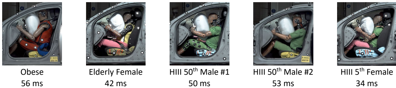
Fig. 27. Still images of the driver seats at time of first head contact with the driver front airbag.
