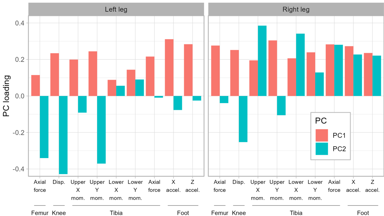
Fig. 5. Crash test metric loadings for the first and second principal components. Note: Disp. = displacement; mom. = moment; accel. = acceleration; PC = principal component.
