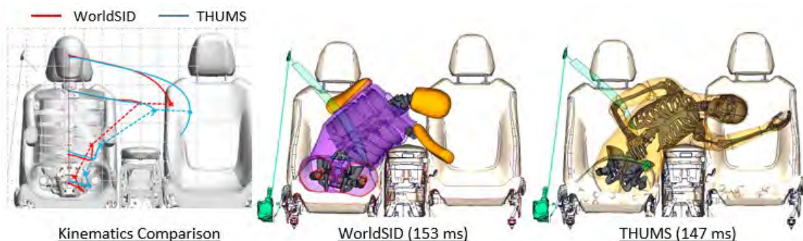
Fig. 10. Occupant kinematics comparison in Pole 75°.
