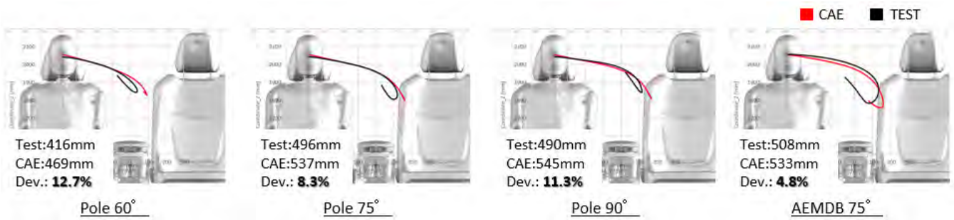
Fig. 7. Head kinematics comparison.
