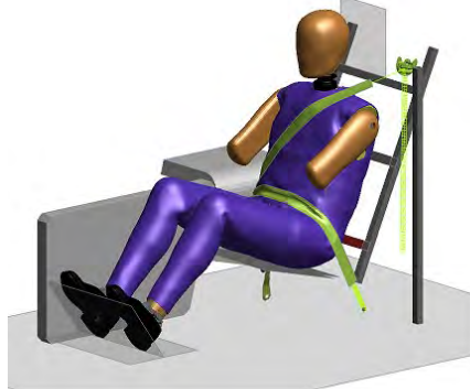
Fig. 1. In-house WorldSID model in the far side environment [14][16].
