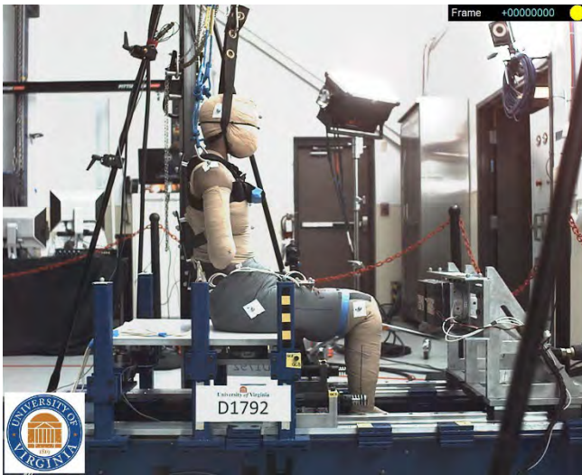
Fig. A1. Example setup of the whole body (WB) test condition obtained from high-speed video.
