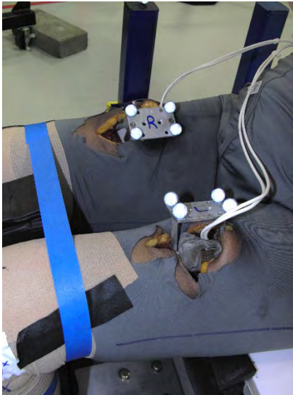
Fig. B1. Lateral “T” cuts made in the specimen to insert femur hose clamp mounts, accelerometers, and motion tracking plates.
