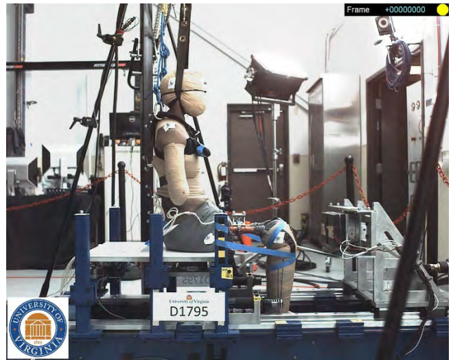
Fig. A2. Example setup of the thigh flesh removed (TFR) test condition obtained from high-speed video.
